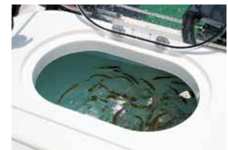
A 42-gallon transom livewell keeps pilchards frisky. The clear acrylic lid eliminates splashing and lets you keep an eye on the liveys.
