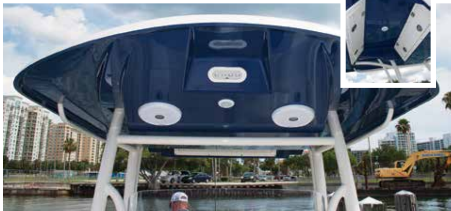
Left: The helm panel is wide enough to accept a pair of flush-mounted 16-inch multifunction displays. Above: An optional two-tone hardtop features built-in floodlights, dome lights and stereo speakers. Inset above: Two overhead boxes offer plenty of stowage for small items.
