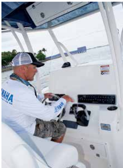
Left: The helm panel is wide enough to accept a pair of flush-mounted 16-inch multifunction displays. Above: An optional two-tone hardtop features built-in floodlights, dome lights and stereo speakers. Inset above: Two overhead boxes offer plenty of stowage for small items.
